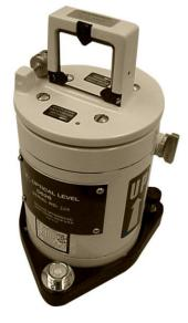
The Model D-626 Optical Level has been designed as an aid to adjust the optical line of sight from an autocollimator until it is precisely level.
