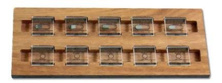
Inspecting and characterizing surface quality of finished optical components e.g.: lenses, prisms, mirrors, reticles, windows and wedges in accordance with MIL-13830, MIL-C-48497 and the new ANSI/OEOSC OP1.002:2008 is easily accomplished using these Scratch/Dig Sample Sets. The samples serve as direct visual comparison standards.
