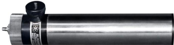
The Model D-691 Laser Alignment Autocollimator is economical enough to be permanently installed in deliverable laser systems or use in house as a Laser Alignment Autocollimator. The instrument incorporates such features as a wide angle field (one degree), average nulling sensitivity of 5 arc seconds, and autocollimating from small reflectors. It comes complete with a power pack.
